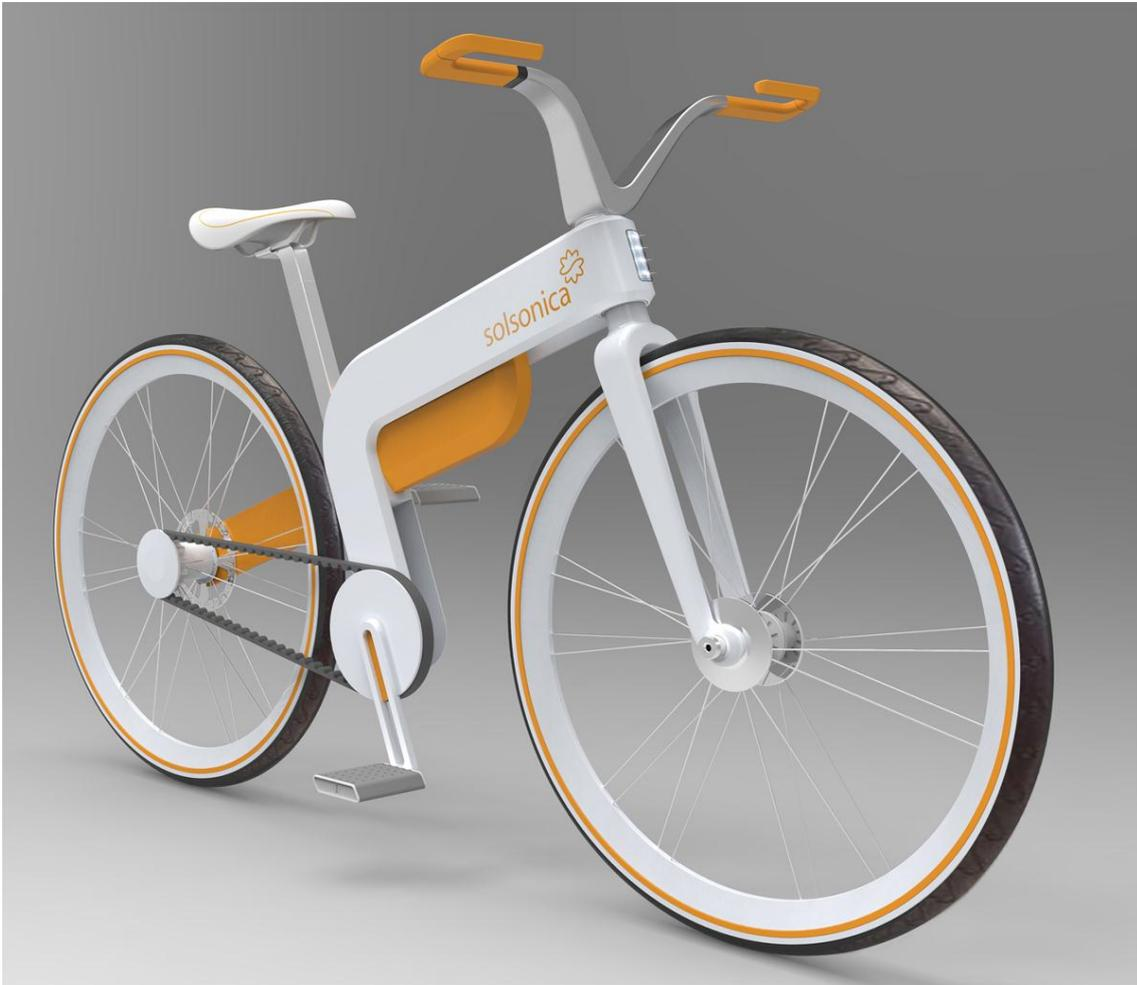
A frame with a "boomerang" shape holds the removable battery pack, placed between the two wheels, gives balance to the bike, with an optimal delivering of weights.
